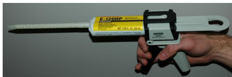
Figure 3.8: Epoxy application system (McAndrew, 2009)
